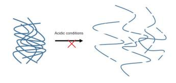
Simplified illustration of membrane degradation when subjected to acidic conditions and strong solvents. The polymeric chains break, leaving larger-than-designed perforations which causes failure.
