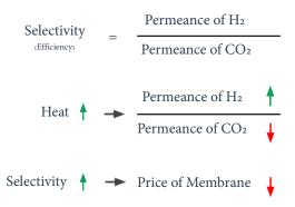
Basic properties of membrane dynamics mechanic present in our membrane. CO<sub>2</sub> is chosen as a benchmark because it has the lowest permeance of any gas. The same equation applies to CO, H<sub>2</sub>S and other gases but selectivity will be even higher.
