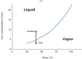
Curve representing the hydrocarbon condensation problem on the residude side of a (typical) hydrogen-permeable membrane. As  $H_2$  is removed from the pressurized feed, the gas becomes enriched in condensable hydrocarbons and its dew point increases.
